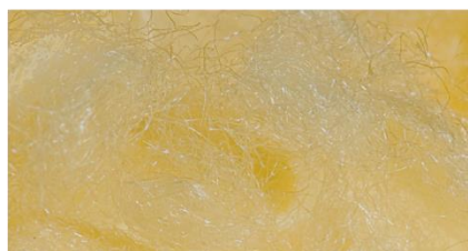
Aqualen™ ion-exchange fiber Fiber diameter: 10 microns Surface area: 1000 cm 2 /g
