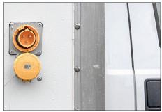
Thumper can provide shore power input if needed and delivers 12,000 Watts of clean sine wave output power with 30 amps of 120V AC. If the shooting set is within 100 feet of Thumper, it includes one 25 FT AC Twist NEMA 30-Amp Pin+Sleeve Extension and two 25 FT AC Twist NEMA 30-Amp Extensions to run from the truck to the set. Thumper ensures your production has the power it needs without any hassle
