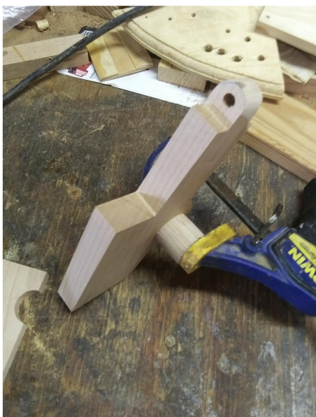
FWD 7: clamping axle housing to body
