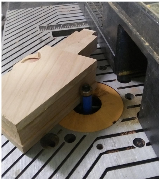
FWD 13: trimming edges of widening panels.
