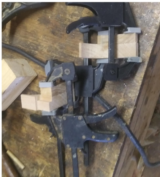
FWD 25: Clamping fender spacer to fenders.
