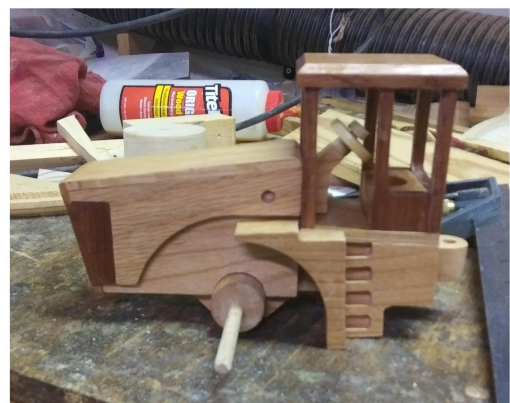
FWD 61: Holes drilled into hood on both sides so that air cleaner and exhaust pipe can be attached.
