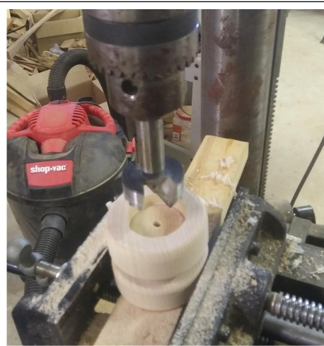
FWD 55. Recess in wheels was formed using a Forstner bit.
