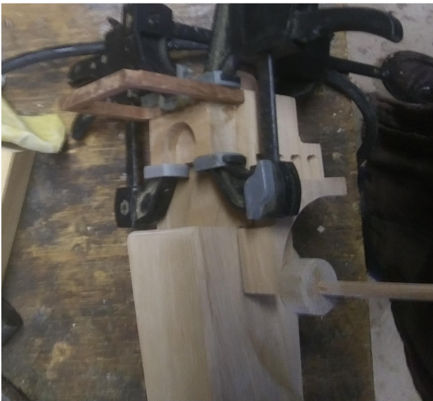
FWD 32: cab back wall being glued to seat
