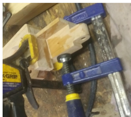
FWD 26: Fender assembly being clamped to tractor body using deck to locate fender, additionally, fender must be square to deck for the adjoining steps to fit.
