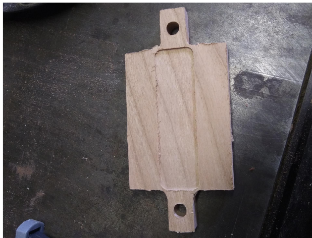
FWD 21: Deck piece as cut by CNC machine.
