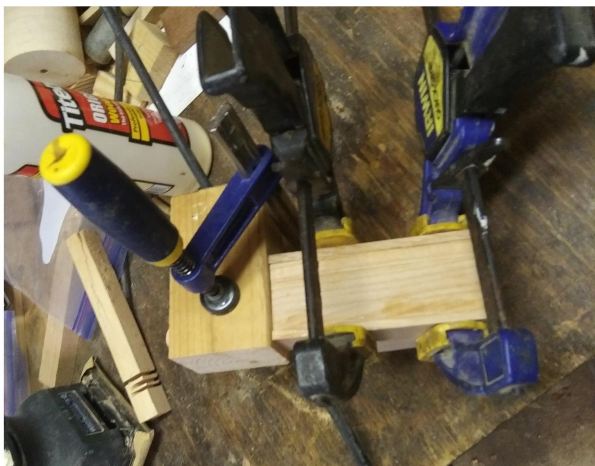
FWD 15: Clamping hood sides using a block clamped to tractor body to locate sides.
