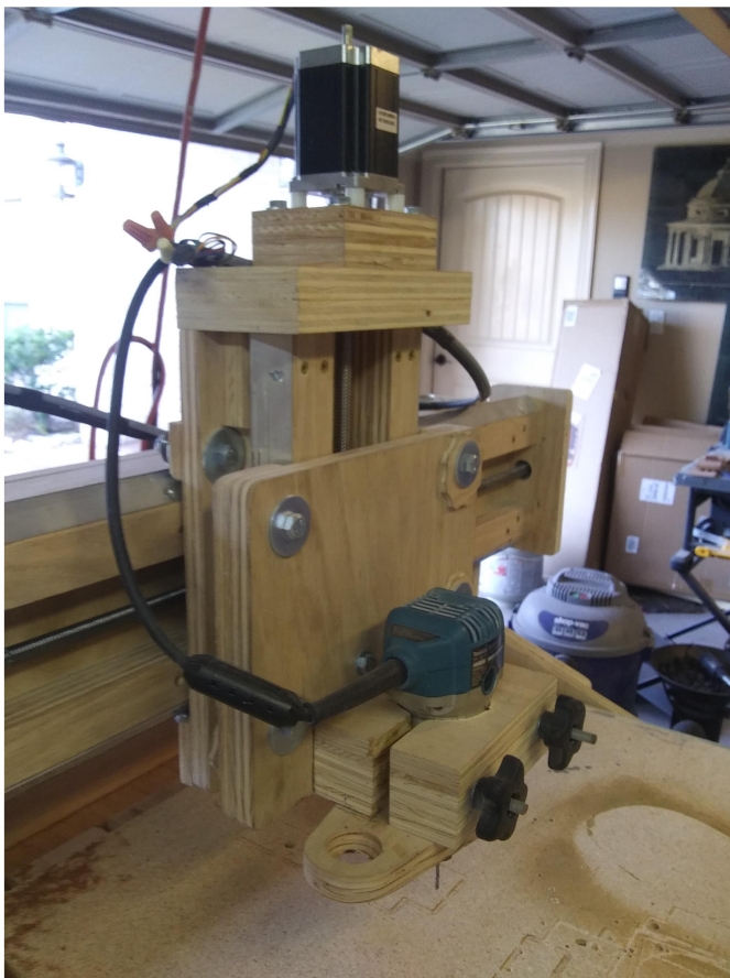
CNC 3: Stepper motor that raises and lowers router and end mill bit under computer control.
