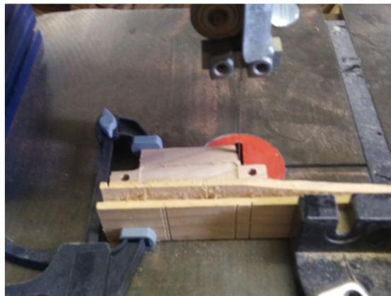
FWD 22: Using band saw with miter gauge to cut off deck tabs
