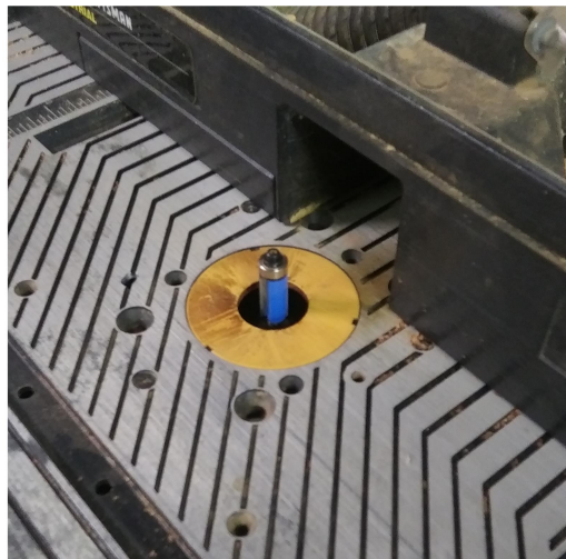
FWD 12: Flush cut bit and router table
