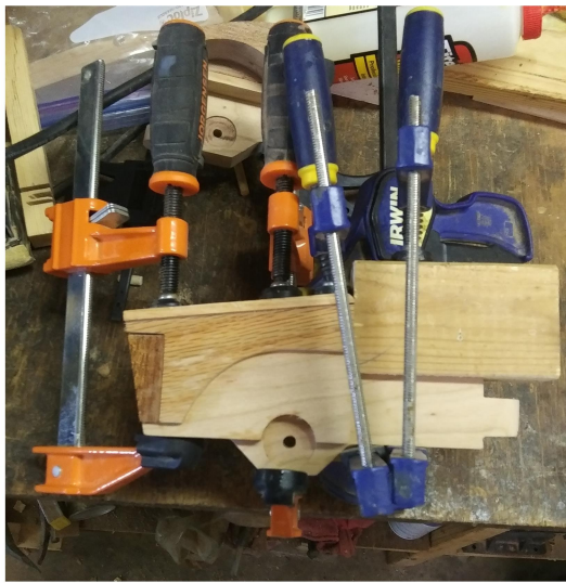
FWD 19. Hood top clamped in place. Block at end of engine compartment used to locate top.
