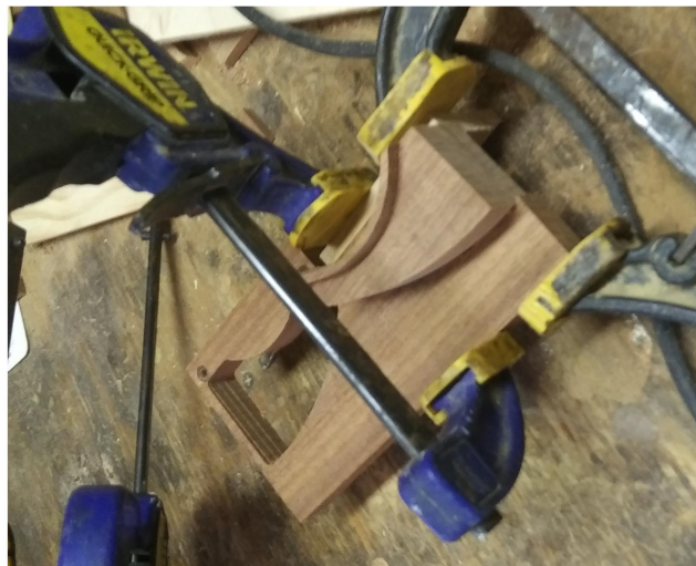
FWD 41: using the cut out blank as a jig to clamp fender/tank assembly to rear deck.
