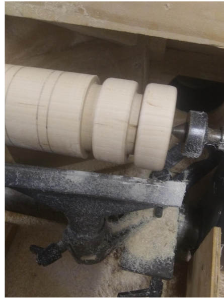
FWD 51. Grooves cut in blank at edge of each wheel. Slight radius put on edge of each wheel.
