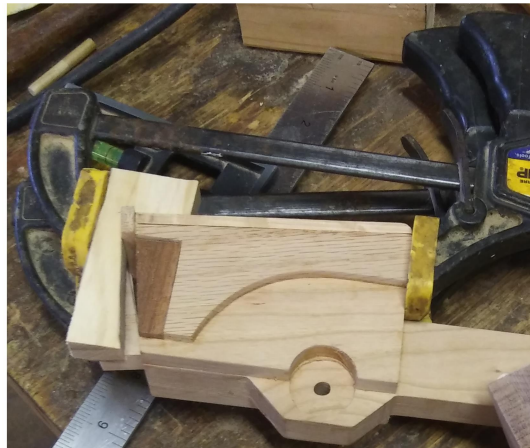
FWD 20: front grill pieces being clamped. Note jig on left used to clamp because of sloped tractor front
