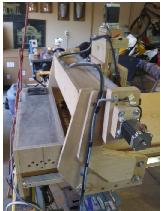
CNC 4: gantry, rail, stepper motors, power supplies, and controller in enclosure.
