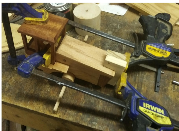
FWD 60 remaining cab assembled and clamped
