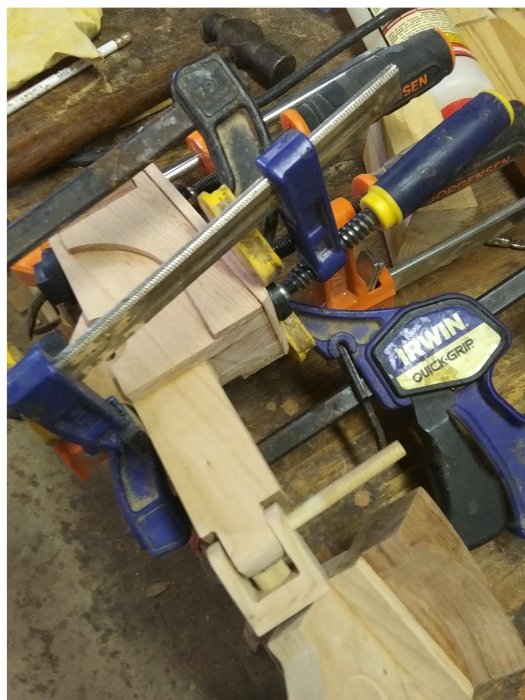
FWD 48: trial fitting of coupler.
