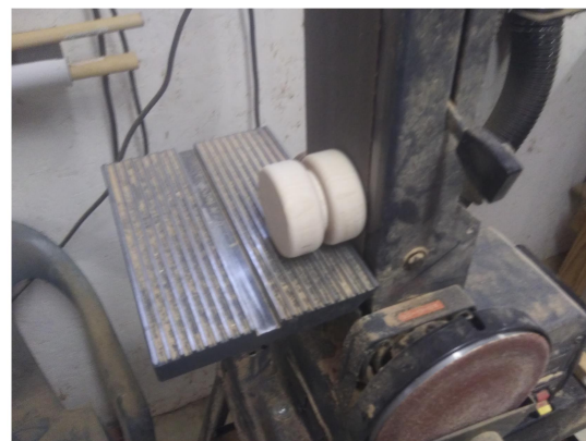
FWD 53: The sawed surface was sanded flush and smooth.
