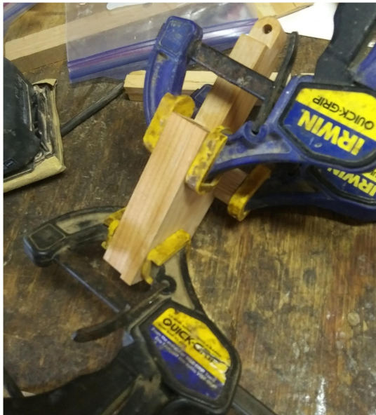
FWD 9: Widening panel clamped in
