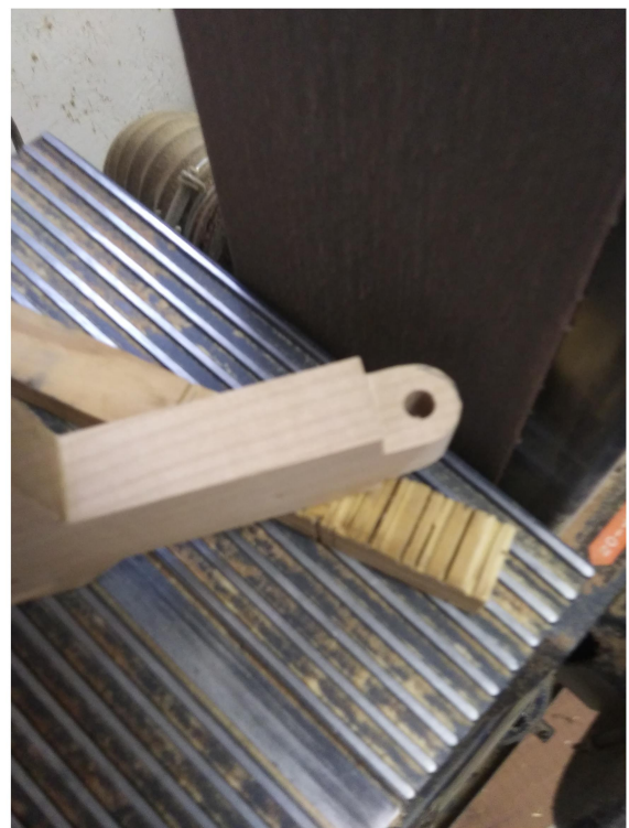
FWD 6: Sanding radius on coupling hitch,
