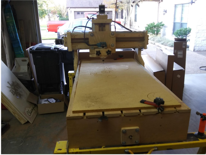
CNC 1: platform and gantries of CNC machine built of wood.
