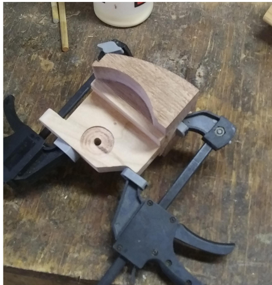
FWD 43: Clamping the fender/tank/deck assembly to the tractor rear body.
