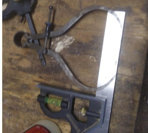
FWD 49: a pair calipers and a scale are used to measure the diameter of the turning.
