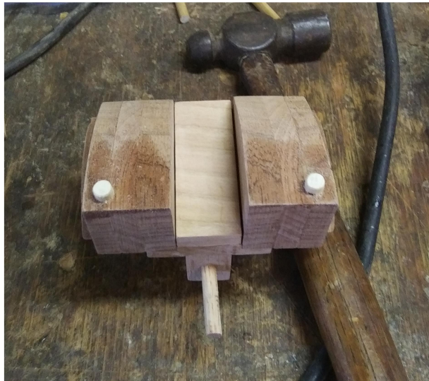
FWD 46: Installed dowel rods
