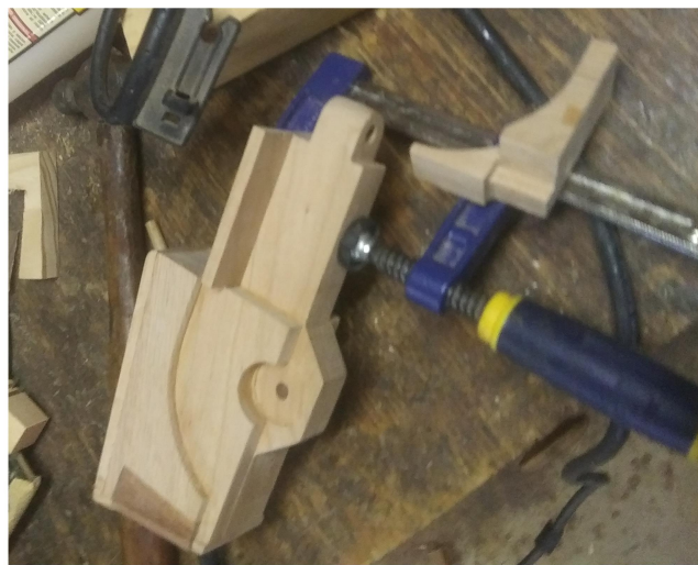
FWD 24 Front deck temporarily clamped in place to locate fenders.
