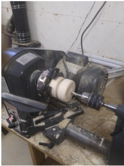
FWD 54: Axle holes in the wheels were bored using the lathe.
