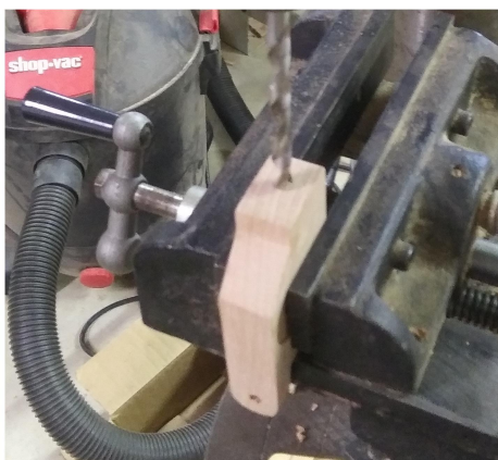
FWD 36: Drilling hold in front rear body where coupling will be attached.
