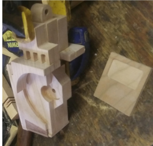
FWD 28: step block on left side and spacer block on right side clamped.
