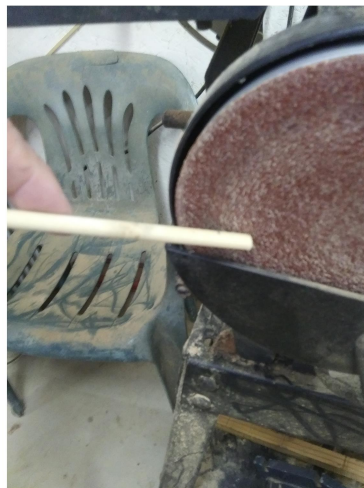
FWD 44: rounding the end of a dowel rod
