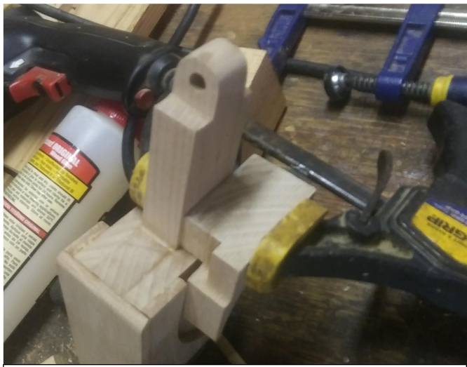
FWD 27. Fender assembly clamped in place and deck temporarily removed to avoid it being glued by excess glue.
