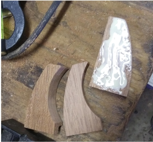
FWD 38: Applying glue to fender/tank pieces
