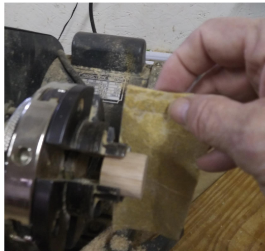
FWD 4: Sanding end of axle housing.
