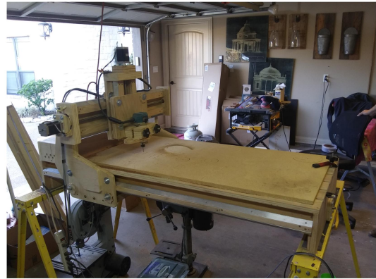
CNC 2: Side of CNC machine showing rails for gantries and stepper motors that move gantries under computer
