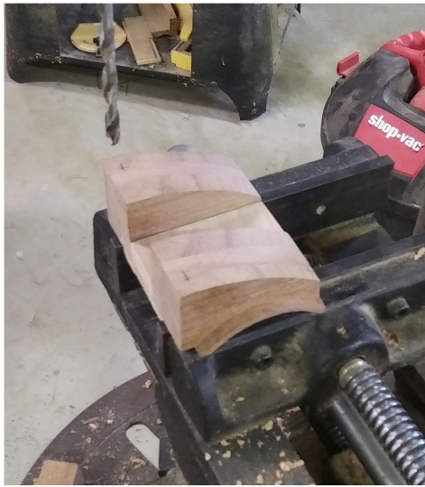
FWD 42. Fender/tank/deck assembly in the x-y vice so that blind holes can be drilled for the fuel tank caps.
