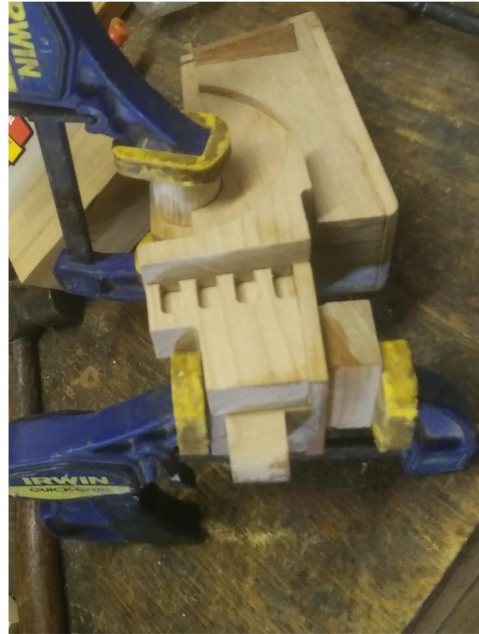
FWD 31. Seat being glued to cab deck
