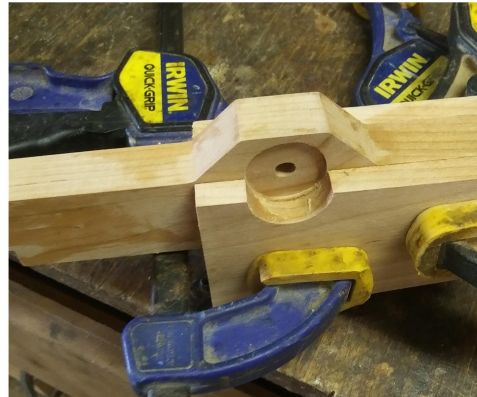
FWD 10: Axle housing removed after widening panels are clamped.
