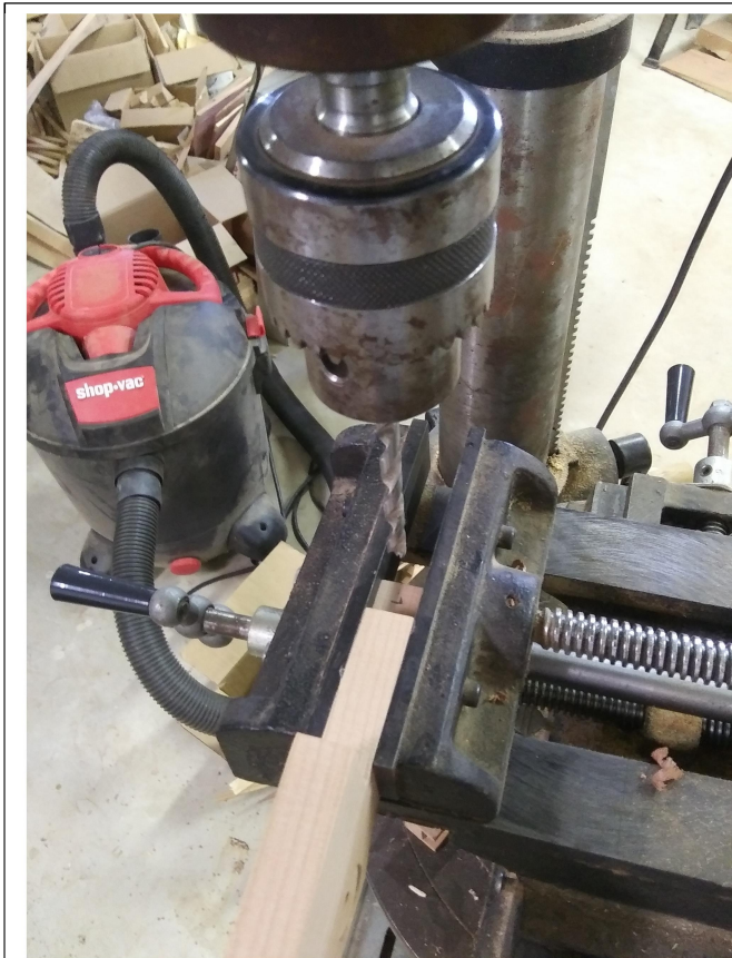
FWD 5: Vice holding tractor body to drill hole for coupling hitch.
