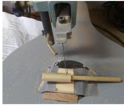
FWD 47: Cutting off retainers with scroll saw.
