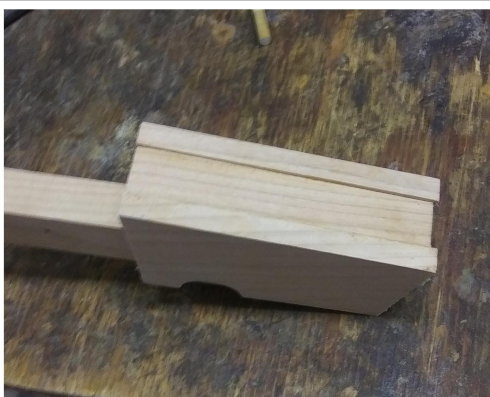
FWD 11: widening panels glued to front body. Note projected edges.
