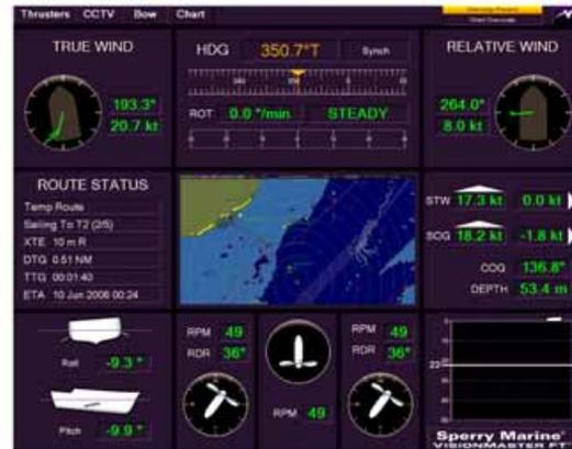
The VisionMaster CID shows critical navigation sensor data in a clear, easy-to-read format, and can be integrated with VisionMaster options such as CCTV.
