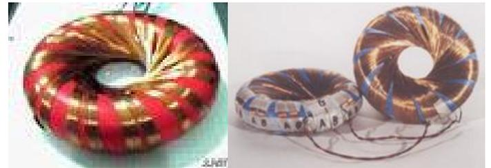
Fig 3a,b. Sample Rodin coils [4,5]
