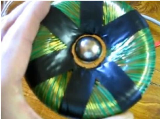
Fig 5. Levitating magnet above a Rodin coil [7]
