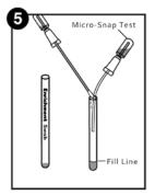
Transfer 100ul or 3 drops from Enrichment swab to Micro-Snap test.
