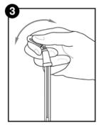
Bend bulb, snapping the snap valve rod and squeeze to release and mix sample.
