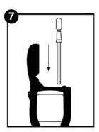
Insert into luminometer and read results.
