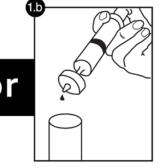
Filter sample through a 0.45 µm (micron) syringe filter.
