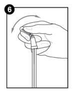
Bend Micro-Snap bulb to break Snap-Valve rod and squeeze bulb 3 times. Incubate for 10 minutes at 37°C.
