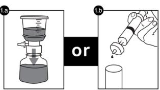
Filter sample through a 0.45 µm (micron) filter.
