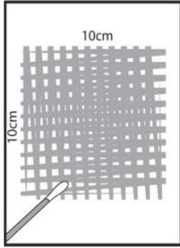
**Regular surfaces:** Swab a 10 x 10 cm (4 x 4 in) square on the test surface, making a criss-cross pattern as shown.
