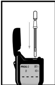
Open the lid on the SystemSURE Plus luminometer, and insert the activated UltraSnap device into the reading chamber. Close the lid.
