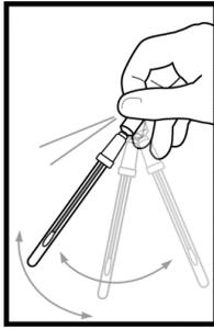
Gently shake the device with a side-to-side motion for 5-10 seconds, bathing the swab bud in the liquid-stable reagent. The test is now activated and the bioluminescence reaction is taking place. For optimal results, the reading should be taken on the SystemSURE Plus luminometer within 30 seconds of activation.
