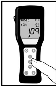
Taking care to hold the unit upright for an accurate reading, press "OK" on the SystemSURE Plus to initiate measurement. Results are displayed on the screen in 15 seconds.
