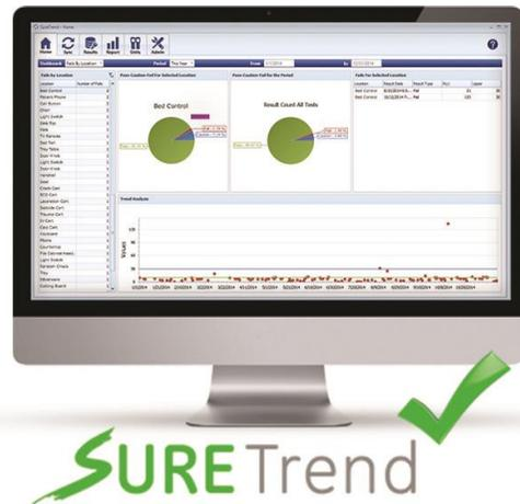
By default the SureTrend software assigns a pass limit of 10 and fail limit of 30 when you add a new location. Assign the correct limits to each location determined in Section 2.1 or 2.2.
