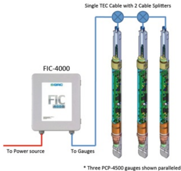
Figure 3: A single digital (FSK) surface interface board supporting multiple gauge communication with up to 6 communication channels.
