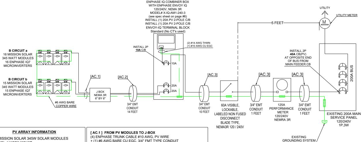
31 MISSION SOLAR 345W SOLAR MODULES MODEL # MSE345SX5T 31 ENPHASE IQ7 MICROINVERTERS MODEL # IQ7-60-2-ACM-US NUMBER OF BRANCH CIRCUITS: 2 NUMBER OF MODULES IN BRANCH CIRCUITS a: 16 NUMBER OF MODULES IN BRANCH CIRCUITS b: 15 MAX WATTS STC: 16 \* 345W = 5520W
