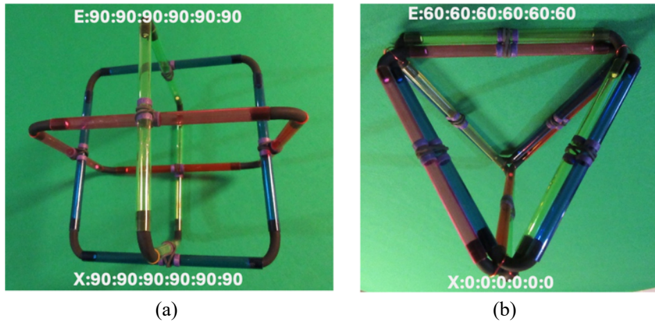
Figure 7: The X-motilitY Structure natural geometric states, (a) the X component with elastic band at 90 degree forming a hexahedron, X-motilitY neutral state (b) X-motilitY in tetrahedral state.
