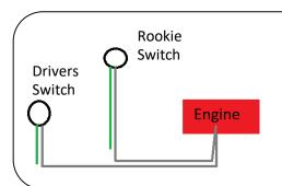
Install Rookie switch on top of car and run one wire from the switch to the engine lead (same as drivers compartment switch).
