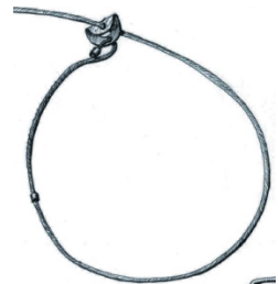
Figure 7. The maximum and minimum loop size for cable restraints is easily measured by circumference. The minimum loop stop is set at 8 inches and the maximum loop stop is set at 38 inches from the reverse-bend washer end of the cable. This results in a loop no smaller than 2½ inches in diameter and no larger than 12 inches in diameter.
