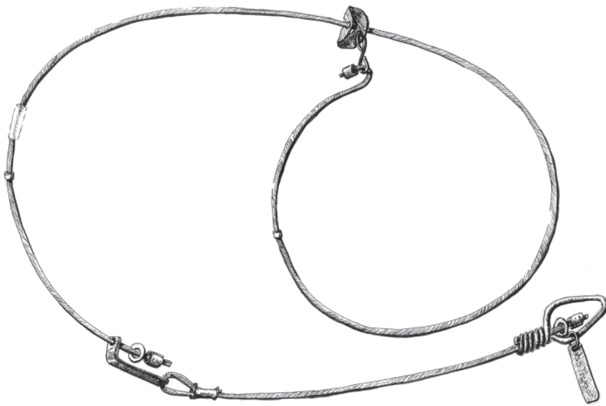
Figure 23. Cable Restraint–J hook: A complete cable restraint equipped with a J hook breakaway.
