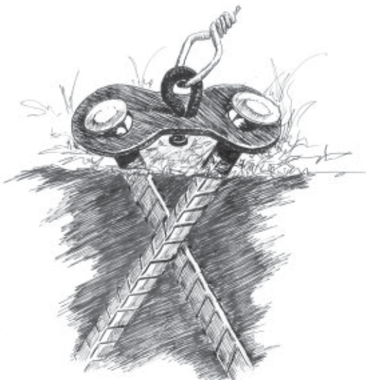
Figure 28. Double stake device: Commercially made double-stake devices allow for ease in connecting the restraint. Note the double swivel action.
