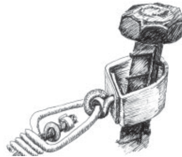
Figure 16. End Swivel + Box Swivel: An end swivel, in combination with a box swivel is recommended.
