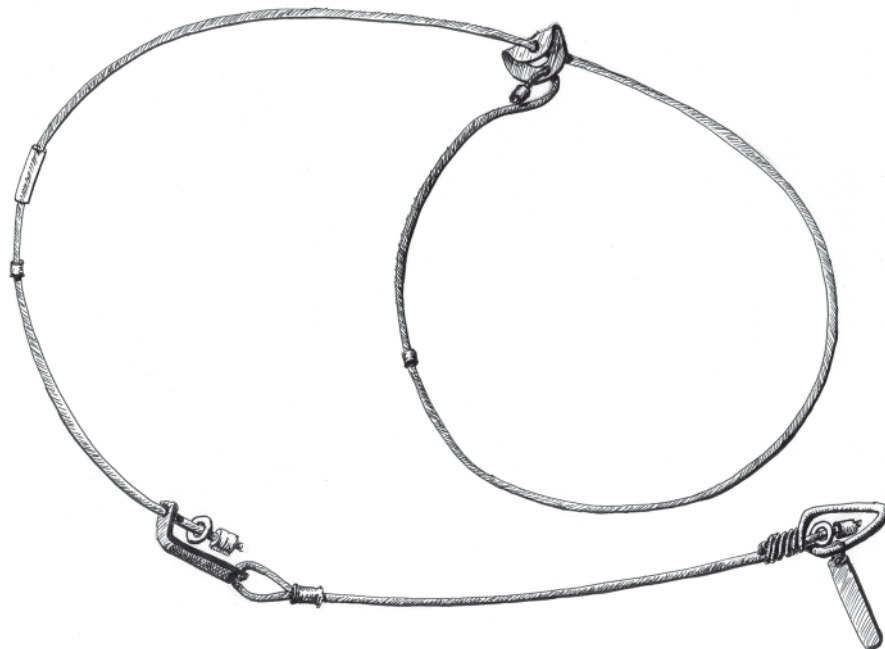
Figure 24. Cable Restraint–ferrule: A complete cable restraint equipped with a ferrule breakaway. This system requires a specialized tool needed to crimp the ferrule to the required tension. It is recommended to purchase these ferrule stops already attached to your cable.
