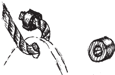
Figure 13. Cable loop with the double end ferrule A double end ferrule provides a secure loop, important when using earth anchors.
