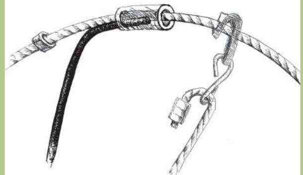
Figure 33. Plastic Collar: Another method of support is with the addition of a short piece of surgical tubing referred to as a collar.
