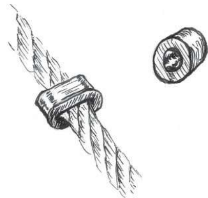
Figure 20. Loop Stop–ferrule: Aluminum ferrules can also be flattened on to the restraint cable and work well as a stop.
