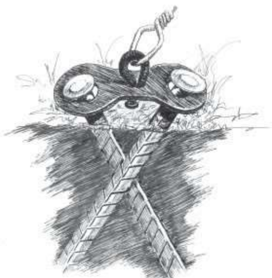
Figure 28. Double stake device: Commercially made double-stake devices allow for ease in connecting the restraint. Note the double swivel action.
