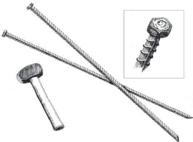
Figure 27. Anchor Stakes: Rerod stakes should be at least 30 inches long, have a nut welded on one end and tapered on the other. A good-sized maul is required to drive stakes of this length!
