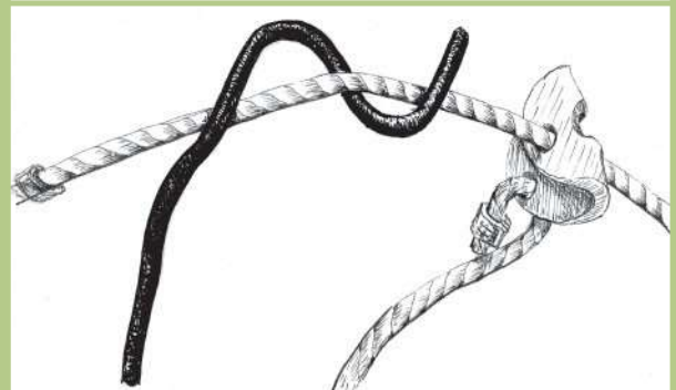
Figure 34. #9 gauge support: Building a small N into the loop support secures the device from easily being knocked down.
