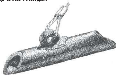
Figure 29. Earth Anchor Tube: Various tubular or flat metal earth anchors work well in unfrozen ground.
