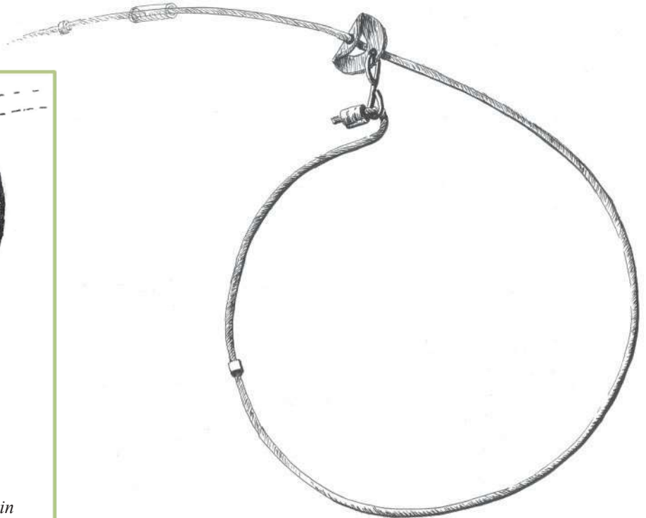
Figure 7. Open Loop: The relaxing lock is a critical part of the cable restraint. The restraint loop is set to allow the animal to enter, which then closes firmly but does not cause discomfort to the restrained animals.
