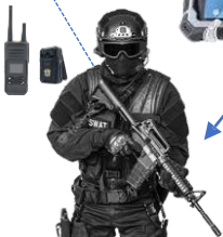
PTT Mesh Radio transmits body camera video and two way audio to vehicle
