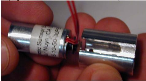
4. Lock the solenoid in place by threading in the 4-40 set screw.
