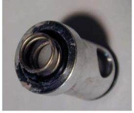
24. Push poppet back and forth inside the valve body to make sure the o-ring does not stick
