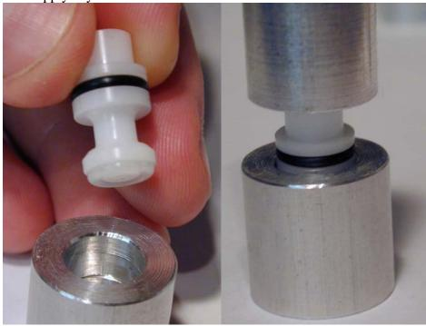
17. Inspect to ensure the o-ring is seated evenly in the groove.
