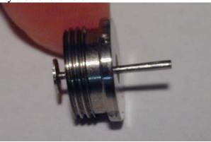
6. Apply a drop of red Locktite or similar high strength thread locking compound to the threads of the orifice plate.
