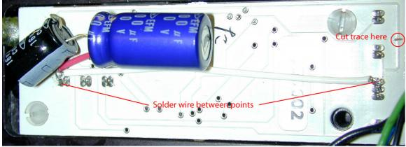
1. Cut the trace as shown in the above figure. This disconnects the 5v bus from the solenoid drivers.
