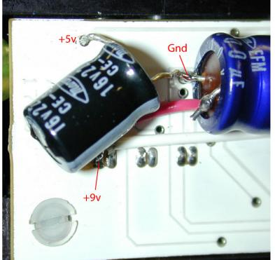
Optional: Connect filter capacitors between 9v and gnd and/or 5v and gnd. Bigger is better in this situation. Use the largest capacitors that will fit inside the grip frame. In this case 220uF was attached to 5v and 1500uF was attached to 9v. Glue the capacitors in place. Electrolytic and tantalum capacitors are polarized, so be sure they are connected properly. Failure to do so can result in a kB!
