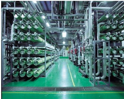
Nanofiltration membrane trains as part of industrial water process for micro-electronics industry
