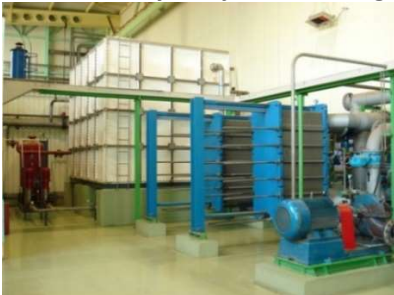
Heat exchanger and ultrafiltration units for industrial process water
