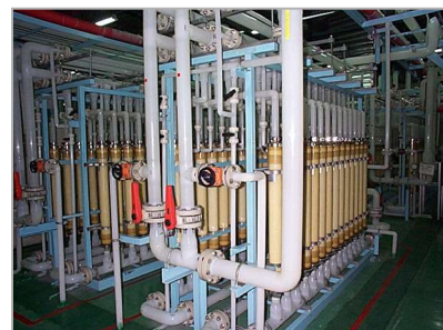
Heat exchanger and ultrafiltration units for industrial process water
