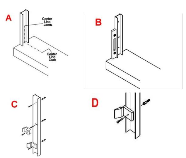
the ZV924 Bumpers (#4) using the 2-#6/32X1/2 Machine screws (#5) keeping in mind that the inside panel will be on the showerhead side of the shower.
