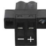
**Note:** The radio fuses will blow if the connected power supply is over voltage, or the polarity is reversed. Two spare fuses are located inside the enclosure (see the 'Spare Fuses' section of the Aprisa SR+ User Manual).
