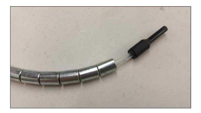
STEP 5 Install the cap over the end of the tube fitting
