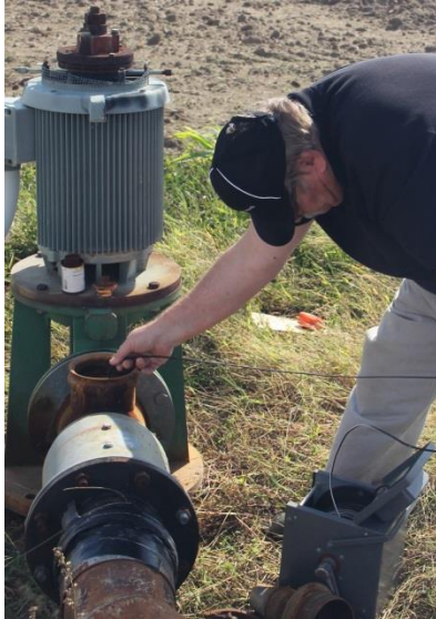
Fig. 5. Sounding SWL by dropping e-line into the column pipe after removing an air relief valve while the pump is off.
