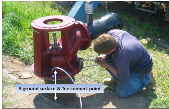
Fig. 10. The length of the air line tubing, L , terminates at where it attaches to the gauge unit, dictating that the measured water surface is measured relative to that point. If the actual distance of water table to some other reference, say ground surface or pump discharge pipe is desired then the vertical distance of these points to the 3-way Tee must be factored in..
