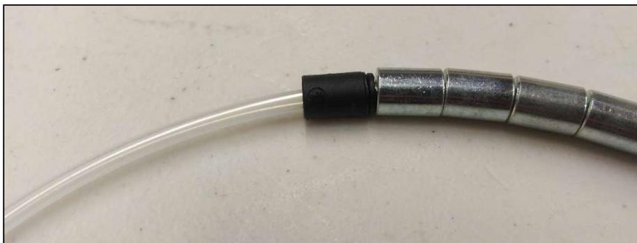
STEP 3 Install the remaining beads over the tubing, as shown below
