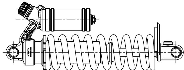
6. Tighten the Preload knob until safety ring and spring are tight and in place
