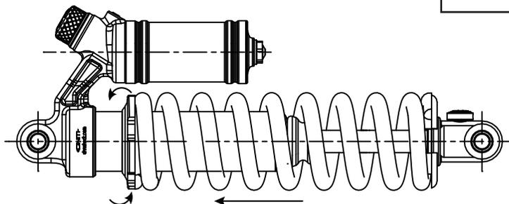
2. Forward the spring until there is space available for remove the safety ring
