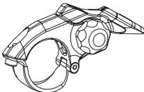
2. For forks with the remote lever adjuster, press the lever down to change the amount of compression damping to the lockout. Note: For more detail installation tips for the TRL or for help in troubleshooting any problems in TRL adjustments, please log on to the RST website ([www.rst.com.tw](http://www.rst.com.tw)) for relative information.
