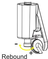
3. Rotate the rebound adjuster as indicated on the sticker to adjust the rebound faster or slower.
