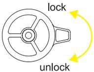
1. For forks with the crown-mounted compression adjuster, rotate the adjuster counterclockwise to change the amount of compression damping to the lockout.
