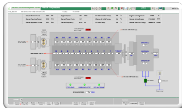
SCADA for Diesel/Gas Engines
