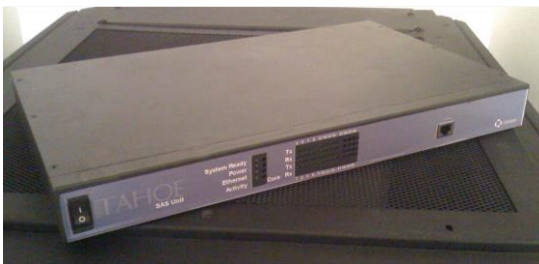
Game Bank Controller for Class III games. Supports SAS 2.0~6.02 with TITO (TSU or Tahoe SAS Unit)
