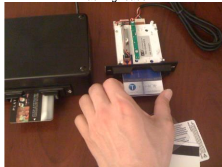
Tahoe Player Tracking card samples shown with internal and external player tracking kits.
