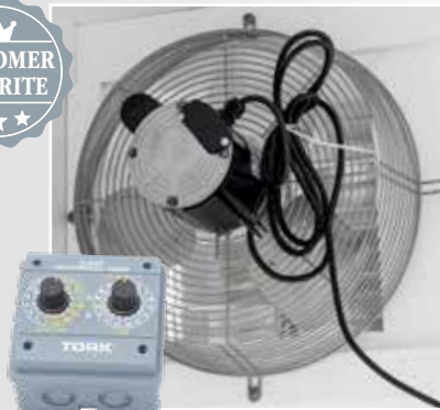
16" 110-V Exhaust Fan w/Aluminum Gable Shutters 1900 CFM 1.35 AMPs With Percentage Timer
