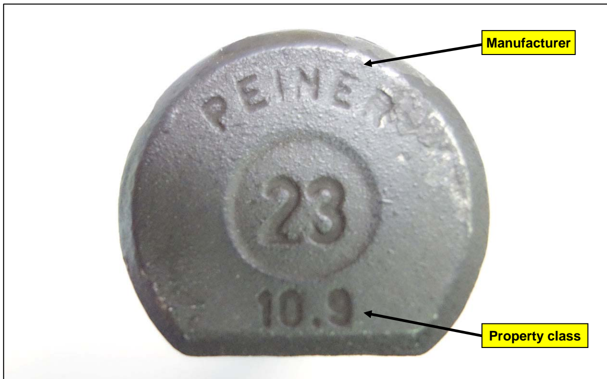
Photograph 6: Identification marks on studs
