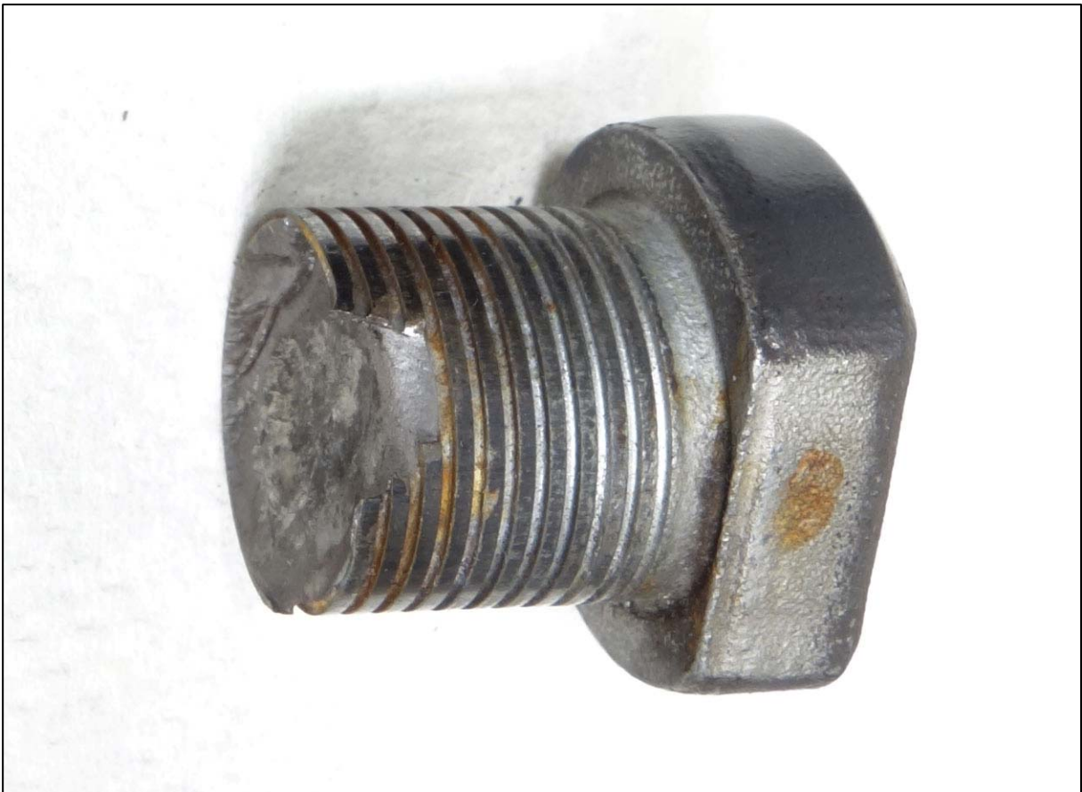
Photograph 8: Broken wheel stud
