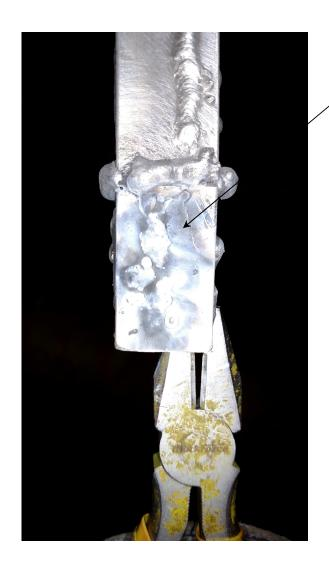
No shielding gas (argon) – weld beads on surface – can't lay down a straight line
