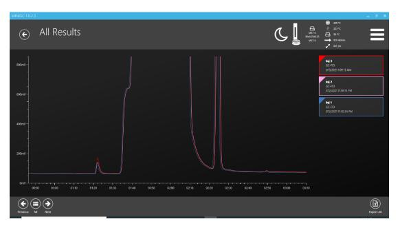
If you don't see a solvent peak (or any other peak), this could mean that the flame in your FID is out. Proceed to the "How To Check if the Ignitor is Working in the miniGC" document to see if this is the issue and if so how to correct it.
