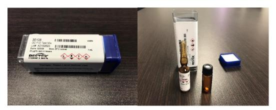
This is the GC-FID Test Mix. It is a standard part from Restek (PN:35108, <a href="https://www.restek.com/catalog/view/33563">https://www.restek.com/catalog/view/33563</a>) that can be purchased from their website. It is also included in the Accessory Kit that comes with the miniGC. It is used to QC every miniGC during checkout at Lucidity before it leaves our facility. And it is the primary means for troubleshooting your miniGC.
