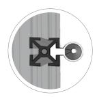
Internal Baffle Eliminates Recirculation and Improves Airflow
