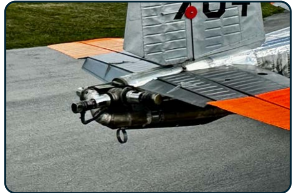
X-14 Rear Puffers / Thrusters (Photo taken 09/06/25)
