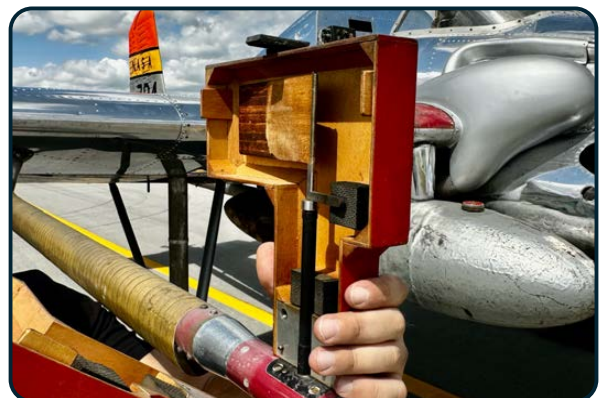
The original X-14 Yaw Sensor Flag Case (Photo taken 09/06/25)
