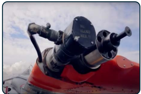
X-14 Wing Puffers / Thrusters
