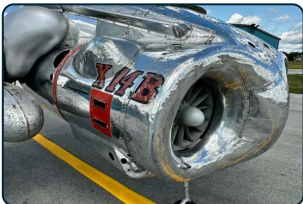
X-14 Right General Electric J-85 engines Engine (Photo taken 09/06/25)
