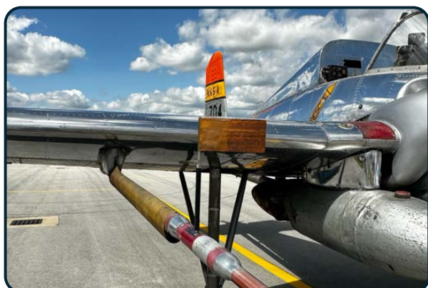
The original X-14 Yah Sensor Flag and Pitot (Photo taken 09/06/25)
