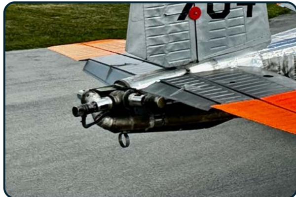
X-14 Rear Puffers / Thrusters (Photo taken 09/06/25)
