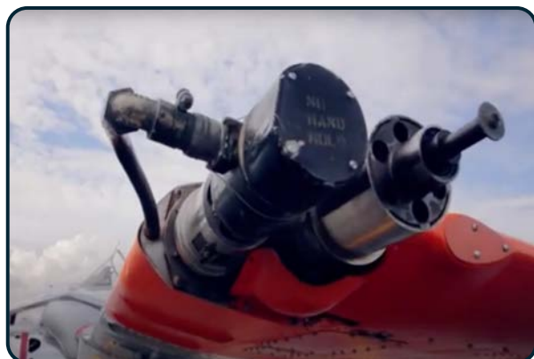
X-14 Wing Puffers / Thrusters
