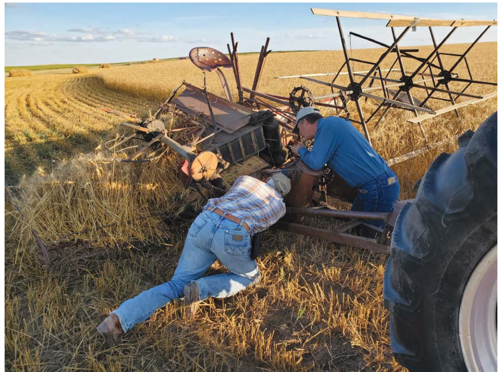
Brian Flatmoe and Wade Hofer work on getting the twine to feed properly on the International Binder. Mice had chewed through the twine in several places.
