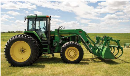
John Deere 7810 MFWD w/740 Classic Loader, (14,000hrs) 19-spd Powershift, 3-hyd, 3-pt, Tires: Front 14.9R30, 18.4-42 480/80R42 Duals, No Lefthand Reverser (Engine Overhaul) (ser#: RW7810P001625)
