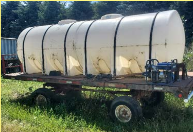
Water Tank Trailer with motor & pump
