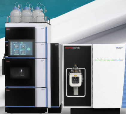
Thermo Scientific™ TSQ Altis™ Plus Triple Quadrupole Mass Spectrometer with Vanquish™ Duo UHPLC
