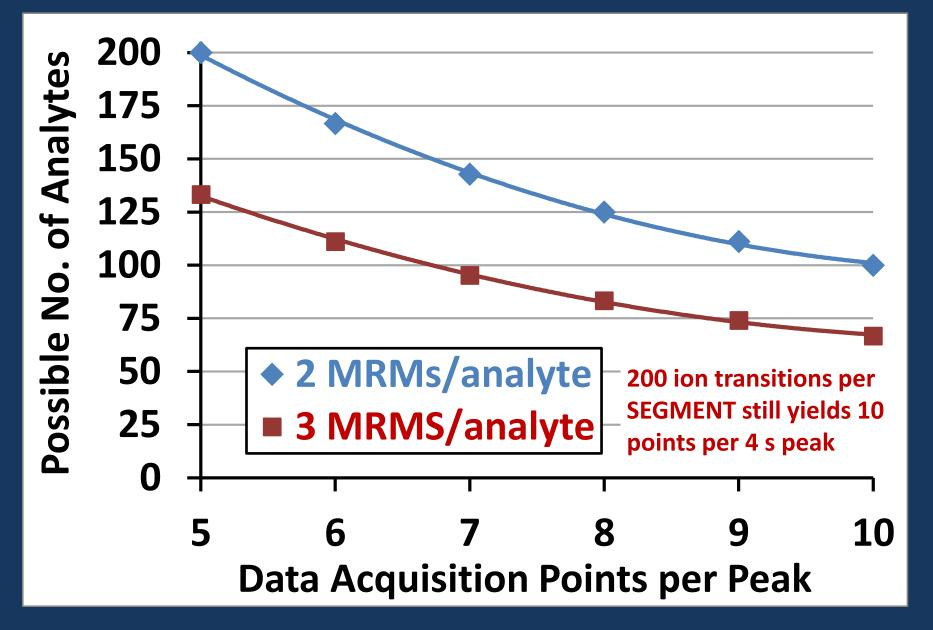
Example of sMRM for 169 Analytes in 9 min 5 points per 4 s peak, 24 s t<sub>R</sub> windows including 20 ms ESI(+/-) switching!
