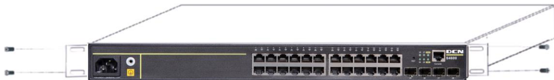
Fig 2-1 Fasten the Brackets to the Switch
