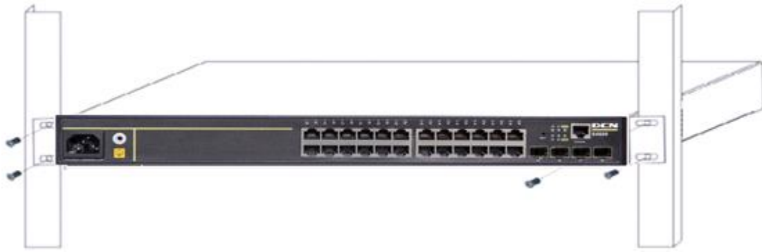
Fig 2-2 Fasten the Switch to the Rack
