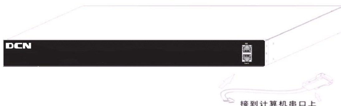
Fig 2-3 Connecting Console to switch
