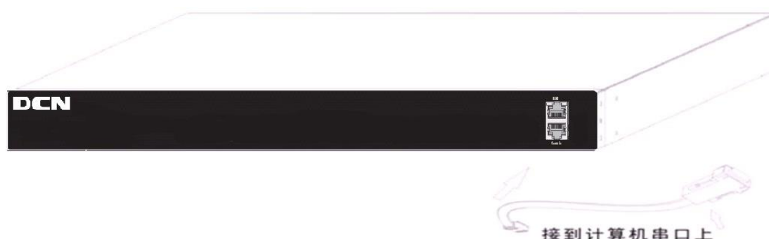
Fig 2-3 Connecting Console to switch
