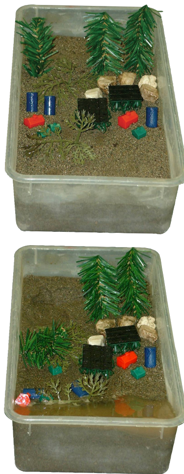
A designed landscape before and after water was applied. Note the destruction on the side of the box with few protective structures.
