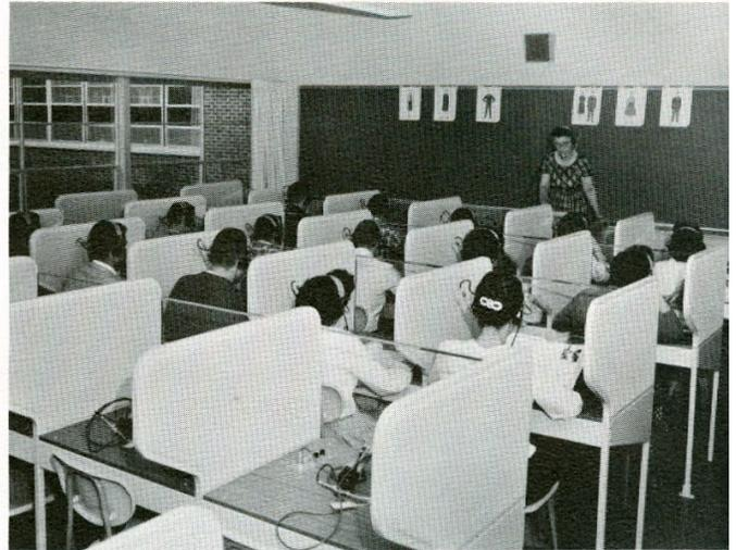
THE LANGUAGE LAB is equipped with a modern functional electronic system to correlate the necessary functions of teaching modern foreign languages. There are 30 student booths equipped with headphones and microphones that in turn are connected with the teacher's master console. The system can transmit simultaneously as many as 5 different programs from the instructor's console to the student booths.
