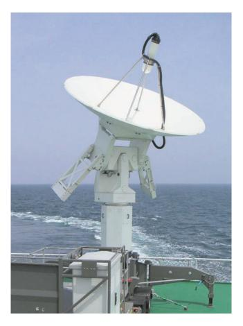
This fully autonomous shipborne antenna system is able to point and acquire targets as low as horizon, even with severe roll and pitch angles .
