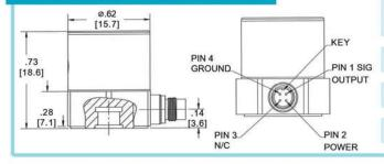
Dual element accelerometer: Piezoelectric and DC MEMS
