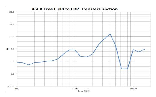
It can be seen that there is an increase of the sound pressure level of approximately 5 dB around 900 Hz and 10 dB around 4 kHz. In order to realistically test the performance of hearing protectors as they will perform on a human head it is important that the size of the test structure resembles the shape of the human head.
