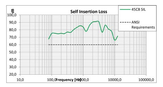
The measurements were performed with a setup as shown in fig.4. with data acquisition and output signal generation software implemented in Labview connected to a NI 4163 USB Dynamic Signal Analyzer. The output signal was broadband pink noise going to a four channel power amplifier driving four full range loudspeakers. The microphone signals from the two artificial ear couplers in the 45CB was connected to a GRAS Type 12AA two channel power supply and from there to the NI 4163.
