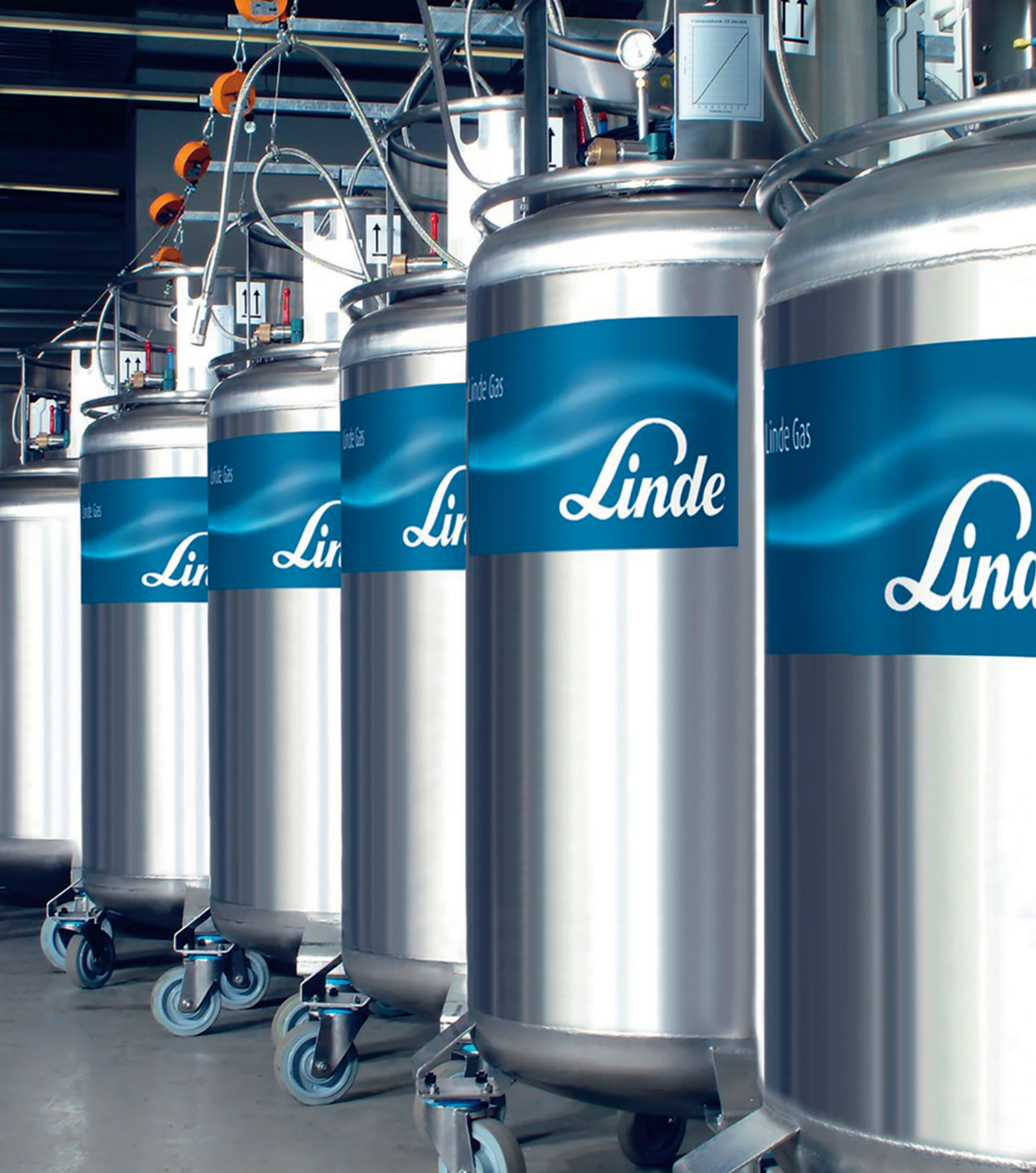
Continuous pressure monitoring of tanks during transport and storage
