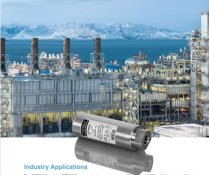
The CPT6020 and the CPT6030 are used when an accuracy of 0.02% or 0.025% of full scale is sufficient. The CPT6020 provides a RS-232 or RS-485 output while the CPT6030 provides a 4-20 mA output. Both have a stainless steel housing, small footprint and calibration interval of 180 days.
