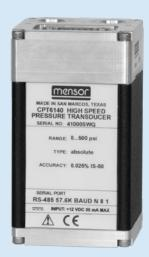
The CPT6140 Is the high speed version in the 6100 series of transducers. It has a pressure output rate of 250 readings per second (50 Hz) and can be configured in a query response mode or continuous "burst" mode. It has a robust aluminum housing, threaded mounting connections, and RS-232 or RS-485 communication options.
